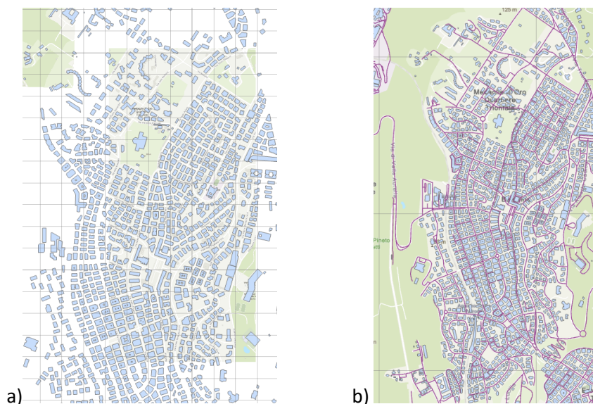
Fig. 22 – a) Creation of barriers (in blue), representing the building areas excluded from the Kernel Density Estimation (KDE) calculation; b) visualization of the road layer where accidents are located
