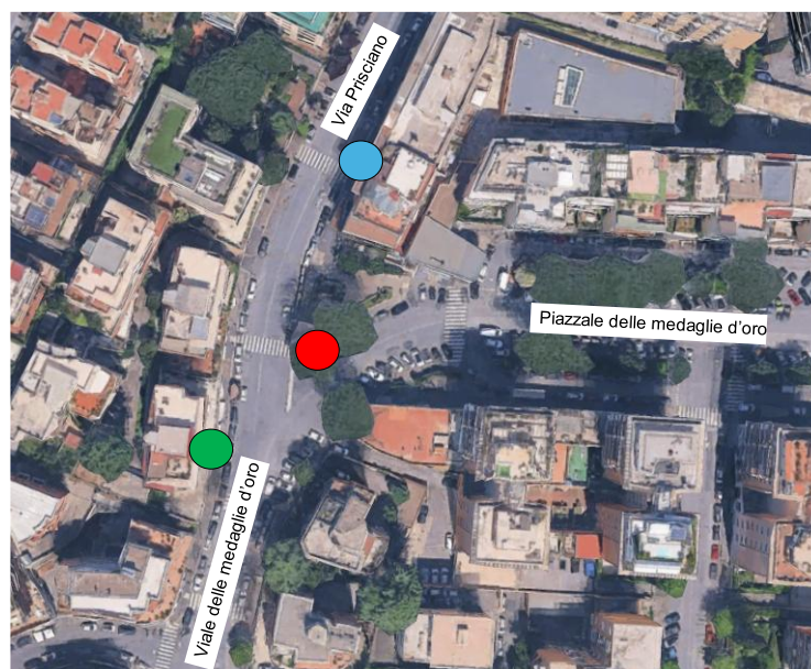
Figure 6 - LiDAR positions at the Case Study intersection
