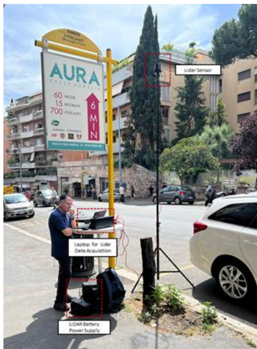
Figure 8 - Field Campaign 1 (Via Prisciano): LiDAR deployment and mobile acquisition station with Prof. Bella (ARCADE PI).
